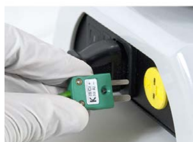
Connection of the external probe, rear side MSH-300i
