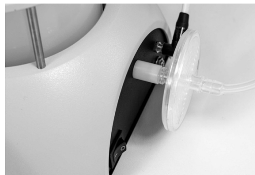
Rear side with ON/OFF switch and hydrophobic microbiological filter
